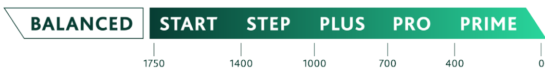
Categorization for carbon steel, in kg CO 2 e per ton of steel.
