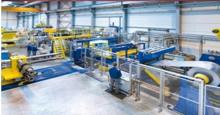
Rolling/ cutting/ slitting of coils
